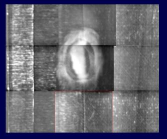
Composite image of repaired area used for monitoring integrity during service
