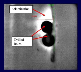
Pulsed thermography used to define damage area for scarf repair
