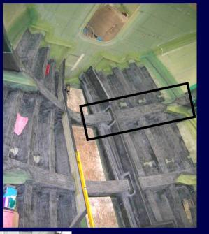
An impact had resulted in debonding of some of the stiffeners from the outer hull
