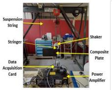
Fig. 1: Experimental set-up.
